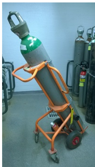
Figure 1. Gas cylinder trolley
