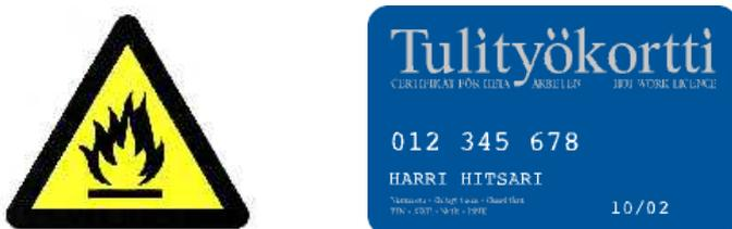
Figure 12 Hot work site sign and hot work card.
