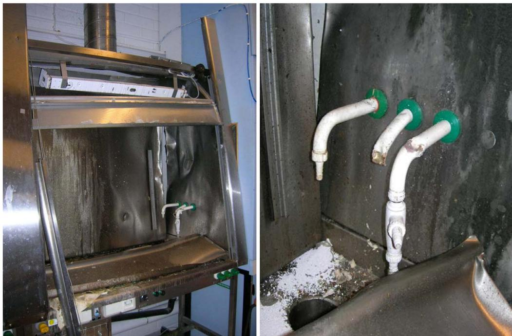
Figure 9 Damages to a vapour hood from a perchloric acid (< 1l) explosion.
