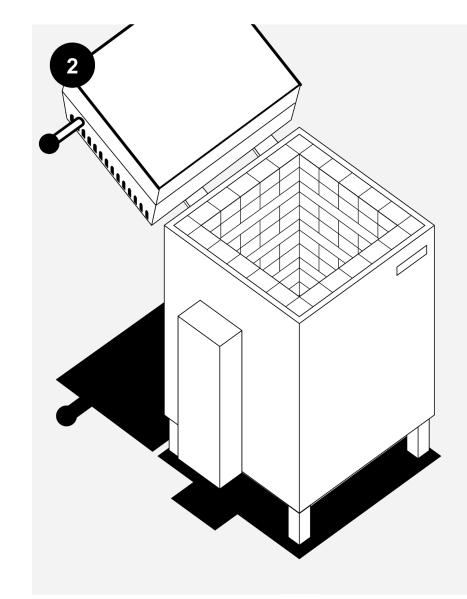
2. The kiln can be loaded when it is room temperature, or cool enough to load safely.
