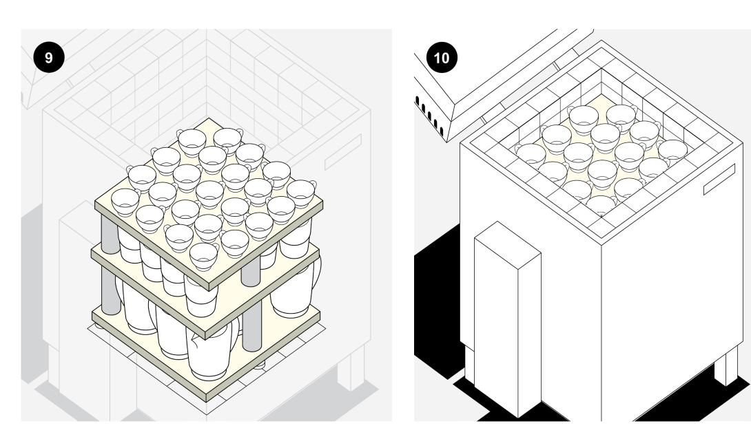
10. Before closing the lid, make sure none of the pieces are too high or they will be crushed.
