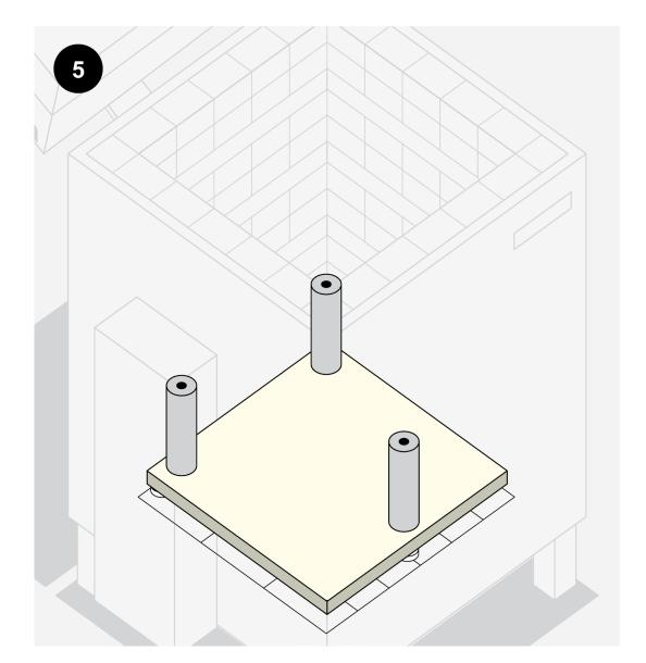
5. The first shelf and posts are placed, continuing the structure of the base of three posts in the same position. The bottom shelf is often a bit taller to help the dispersion of heat throughout the kiln.
