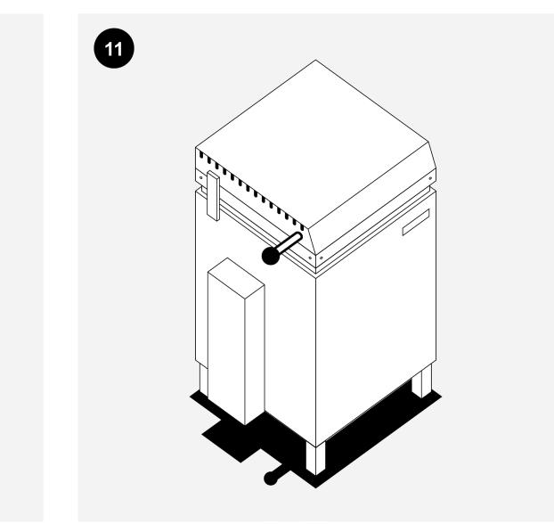
II. Close lid, program and start kiln. Make sure there are no flammable materials in the kiln.
