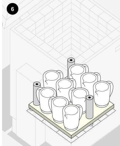
6. Pieces of similar height should be placed on each level, maximizing the area of the kiln to run it as efficiently as possible
