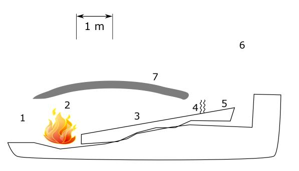
on placement of objects and loading. In the kiln chamber nearest the fire box, work can be completely covered in ash and smoke. It is possible to put ceramic pieces without glaze into a wood kiln, as the very hot build up of ash from the wood will cover pieces with a glaze-like surface.
