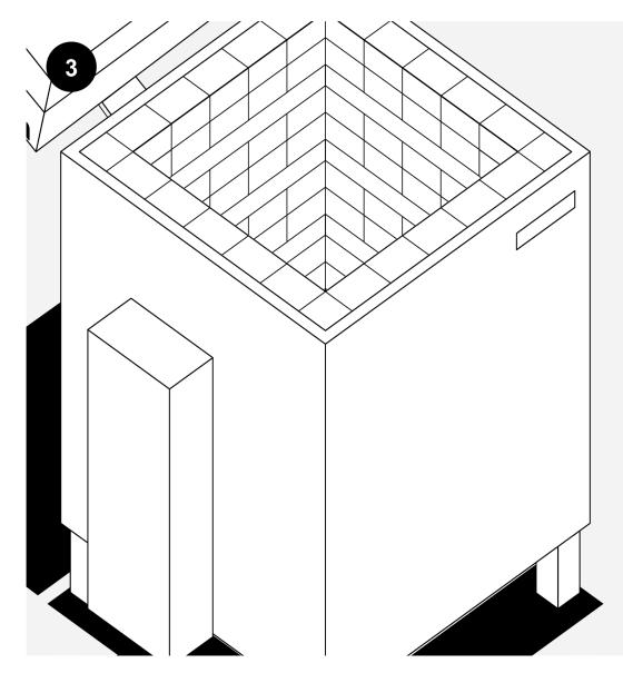
3. The heating elements line the inside of the kiln in rows and there should be no debris or shards on them or other damage.
