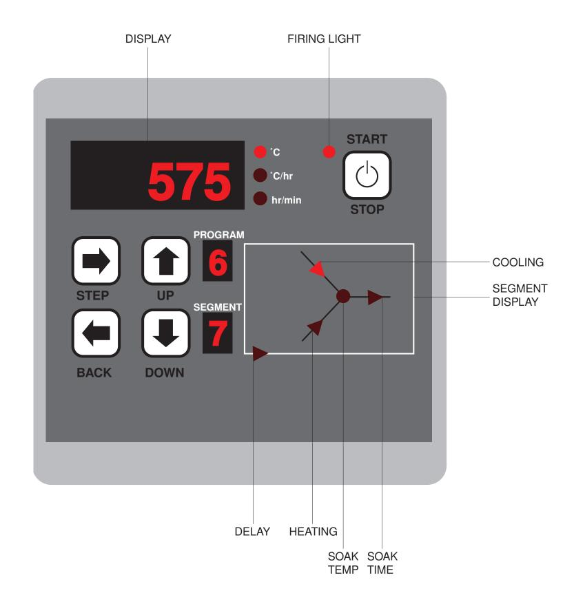
Figure 2: Kiln control pad by Stafford Instruments for Kerako Kilns. Most common at Aalto University, and the diagram shows basic button functions.
