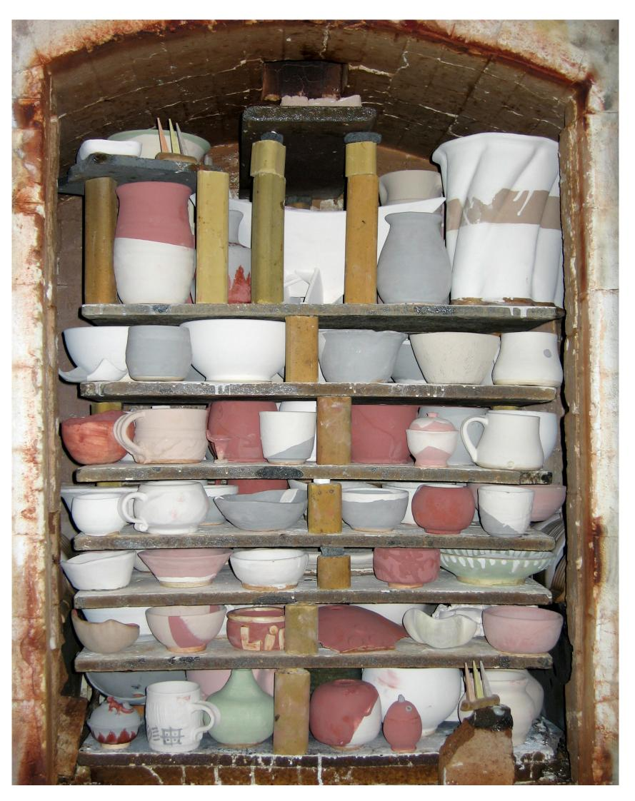
Figure 5: Fully packed gas kiln before firing with cone packs at the top left and bottom right.
