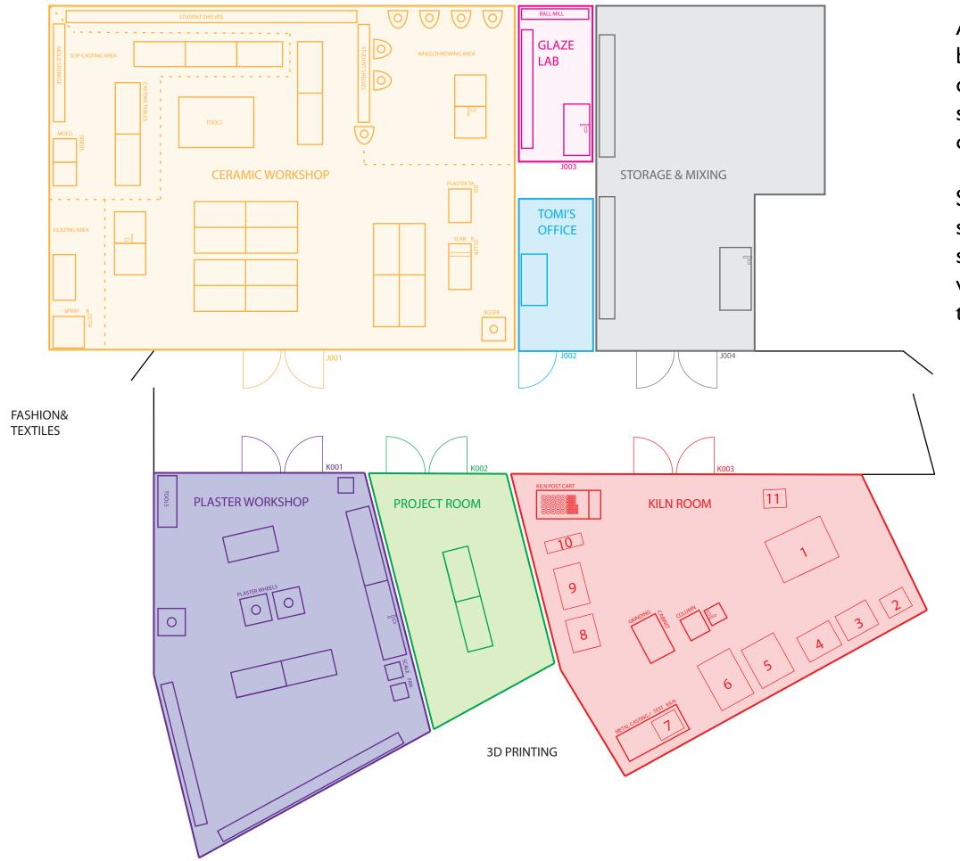
Figure 15: Aalto University ceramic workshop layout. The equipment has been organized in the space to create different areas for different tasks, such as glazing and slip-casting.
