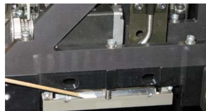
Figure 6-37: Cleaning the roller waste collector
