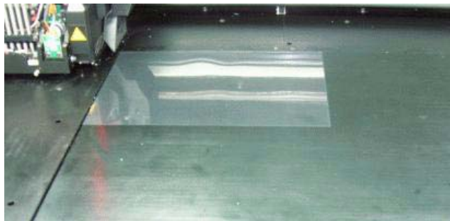
Figure 6-45: Positioning the transparency on the build tray
