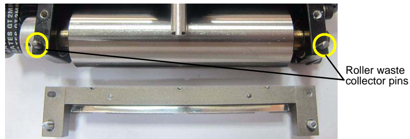
Figure 6-38: Roller waste collector pins
