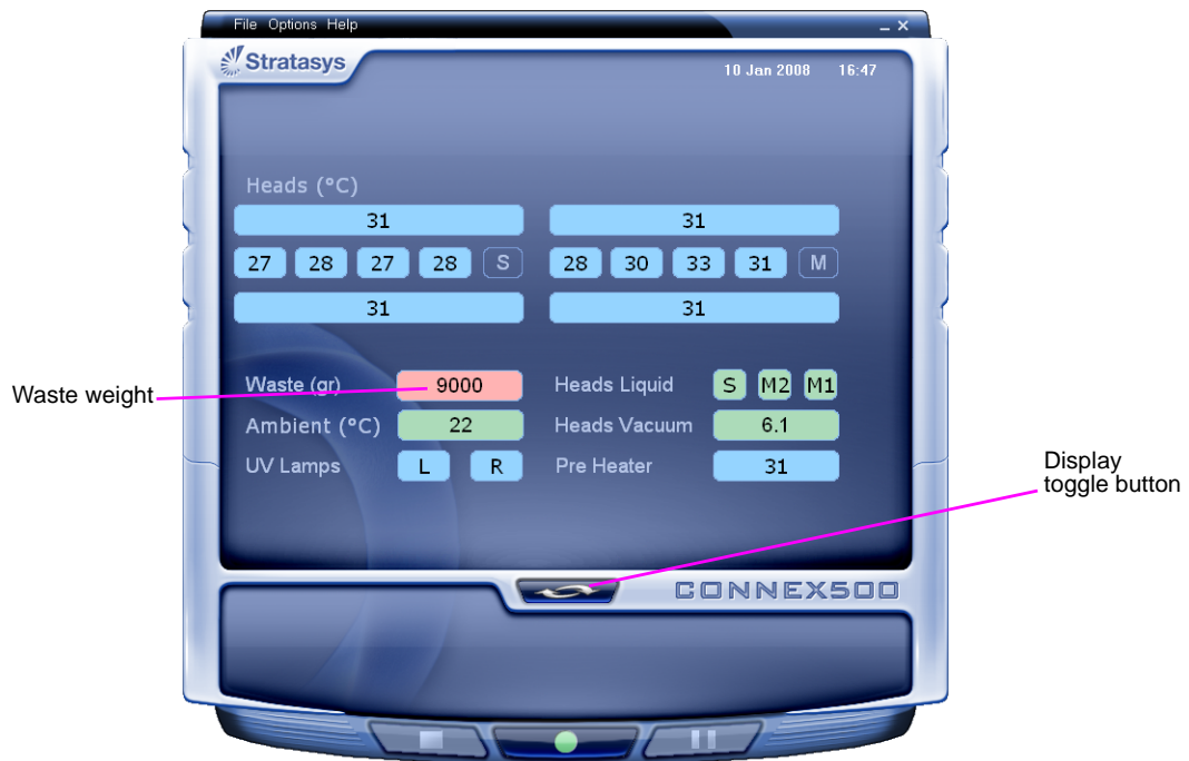
Figure 6-104: Printer interface, showing waste weight (red background indicates operator alert)
