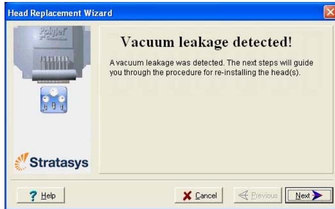
Figure 6-72: Vacuum-leakage warning screen
