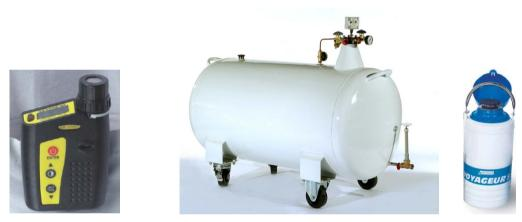
Figure 11 Portable gas detector and two types of cryotanks
