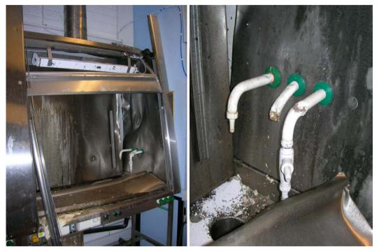
Figure 9 Damages to a vapour hood from a perchloric acid (< 11) explosion.
