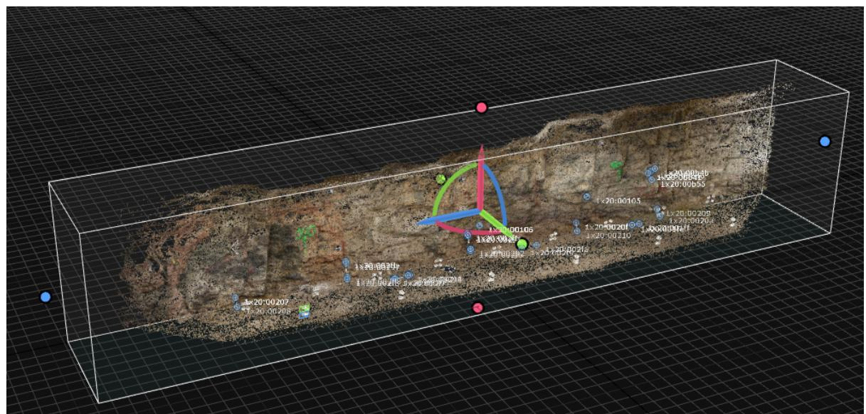
Meshing - Note: This step can only be completed if your computer has an NVIDIA GPU with CUDA cores!!!
