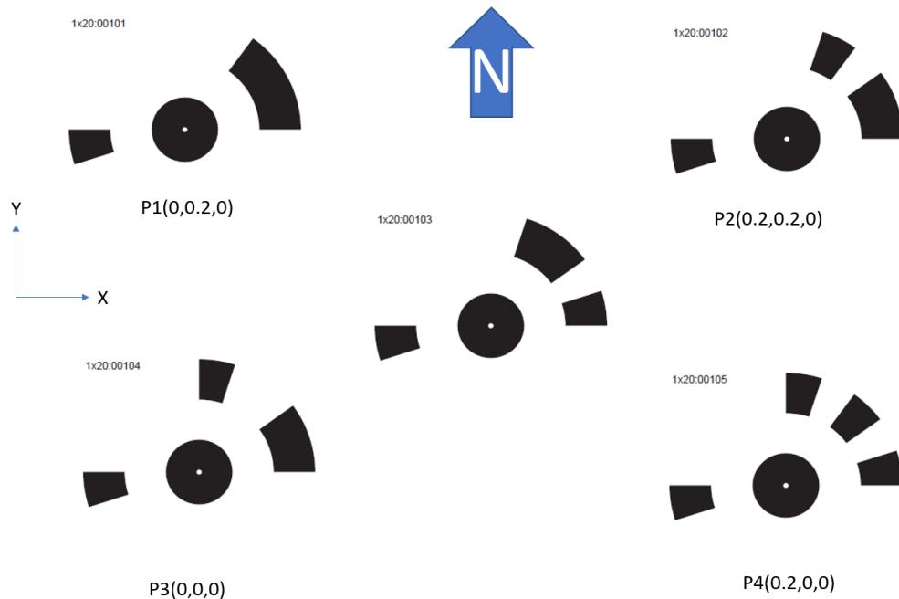
18. Remember to change from tie points to ground control on all the 4 markers on the alignment board.
