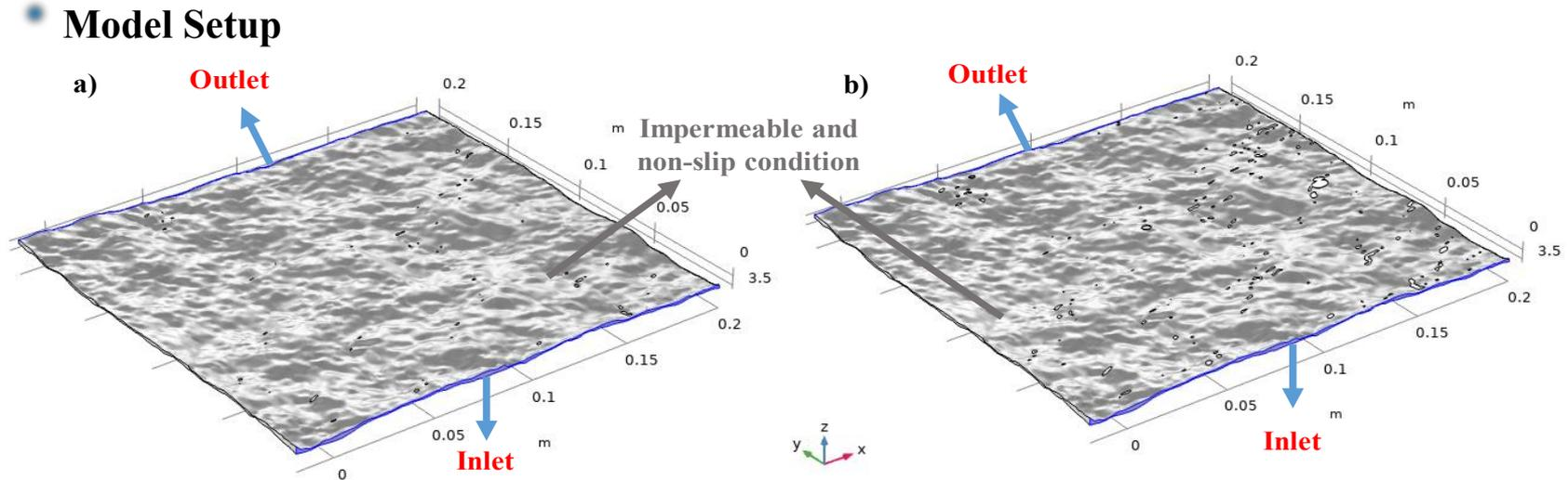
Figure 9. Boundary conditions for flow simulation for the fracture without normal stress (a) and the fracture under 0.5 MPa normal stress (b).
