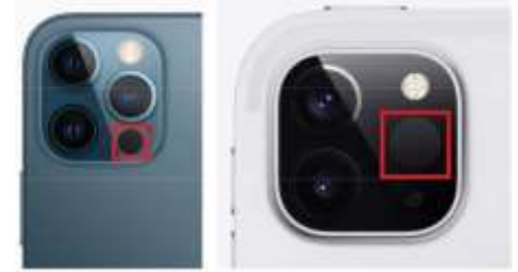
LiDAR sensor location on Apple iPhone Pro 12 (left) and iPad Pro 2020 devices
