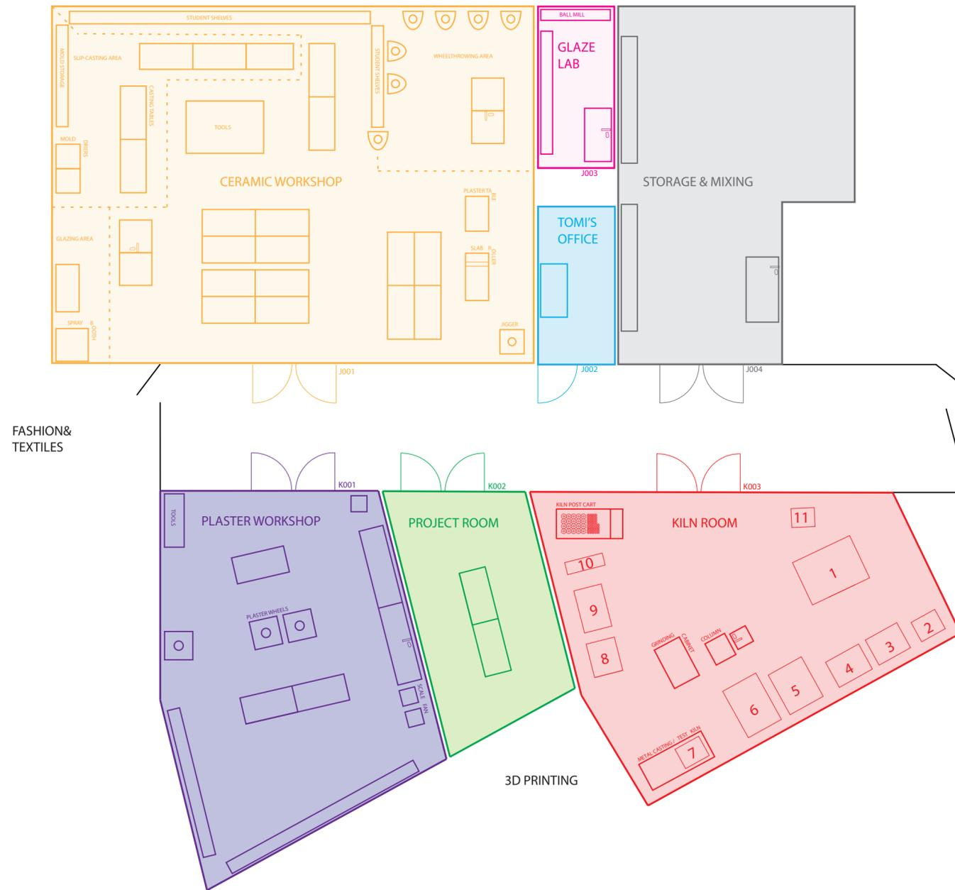
Figure 15: Aalto University ceramic workshop layout. The equipment has been organized in the space to create different areas for different tasks, such as glazing and slip-casting.
