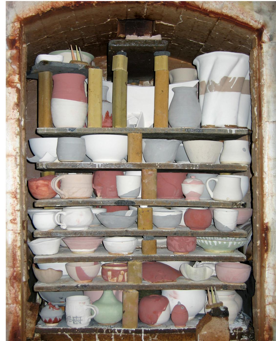
Figure 5: Fully packed gas kiln before firing with cone packs at the top left and bottom right.
