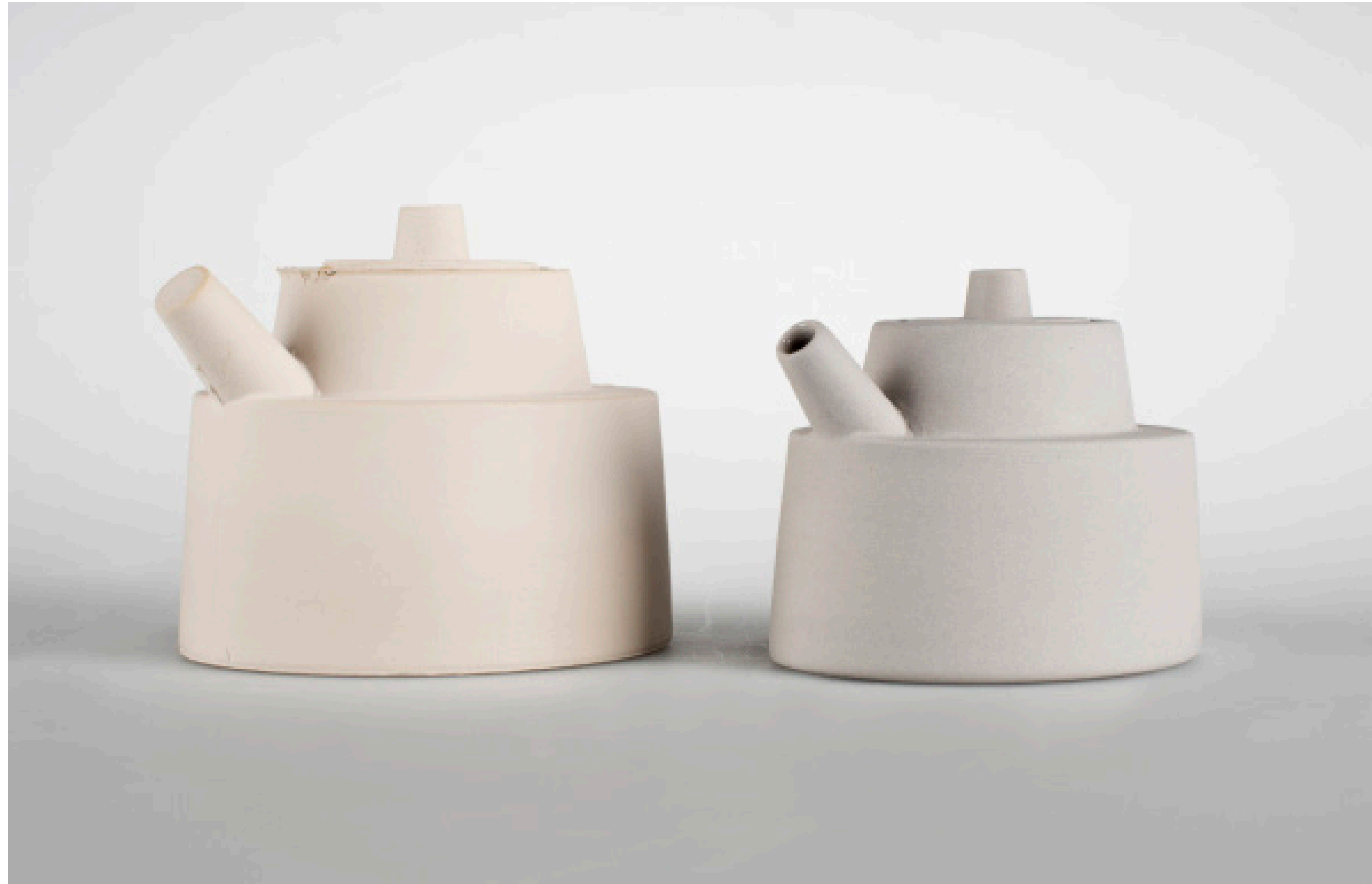
Figure 3. Post-firing changes, such as firing shrinkage, are seen when the unfired and vitrified fired pitcher are compared. Pitcher by Nathalie Lautenbacher
