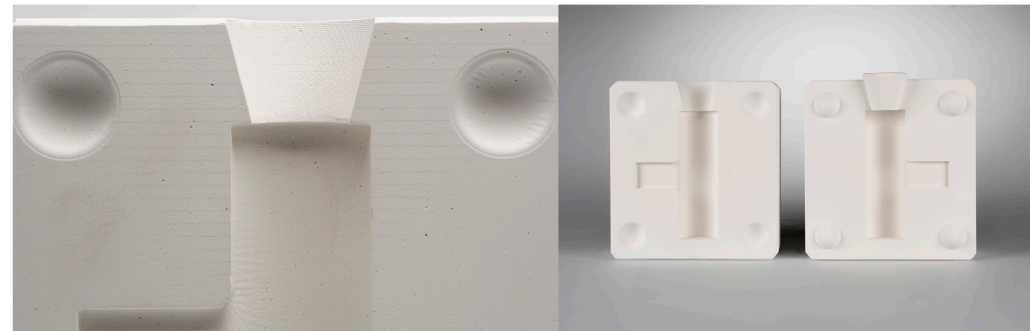
Figure 15. Mold example: Handle mold molded with a CNC milling cutter. Mold Piia Jalkanen
