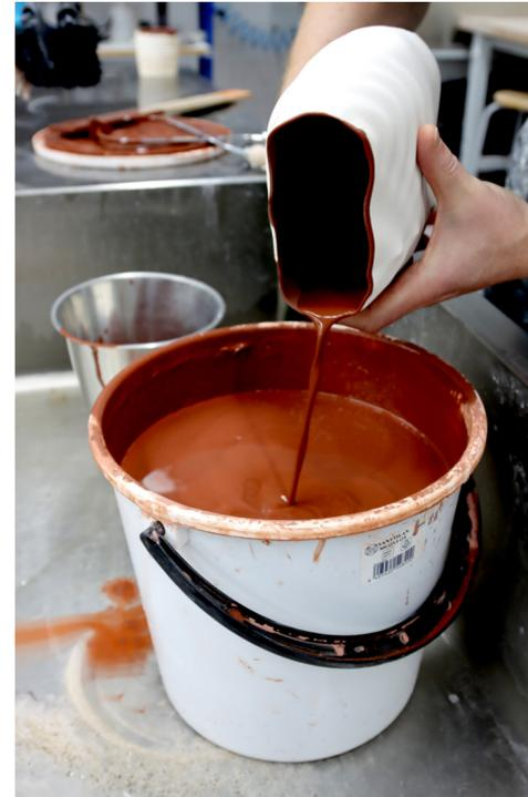
Glaze is poured on the outside or inside of an object. When glazing the interior, the glaze is poured back into the container. The thickness of the remaining glass layer is determined by the speed of work, i.e. the longer the glaze liquid remains inside the object, the thicker the glaze layer. In pouring, the glaze waste is also small when pouring is done above a container and the excess glaze is recovered.
